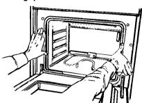
Push against seal area of front frame to push oven into cabinet.
